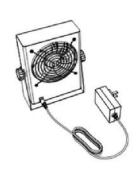
Take out the power adapter from the packing box and connect the ionising air blower. Place the ionising air blower close to the working area (about 150~450mm away from the object with electrostatic to be eliminated), and the air outlet of the ionising air blower must be vertically aligned with the object to be eliminated.
