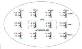
The test data as follows (test distance: 450mm in front, maximum air volume):
