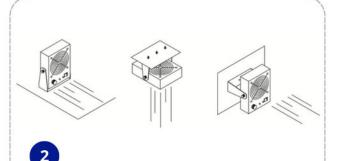
Use screws or bolts to fix on a firm and flat surface (such as a wall or shelf). The angle of ionising air blower can be adjusted by the knobs on both sides of the bracket to achieve the best static elimination effect.
