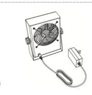
Take out the power adapter from the packing box and connect the ionising air blower. Place the ionising air blower close to the working area (about 300~750mm away from the object with electrostatic to be eliminated), and the air outlet of the ionising air blower must be vertically aligned with the object to be eliminated.
